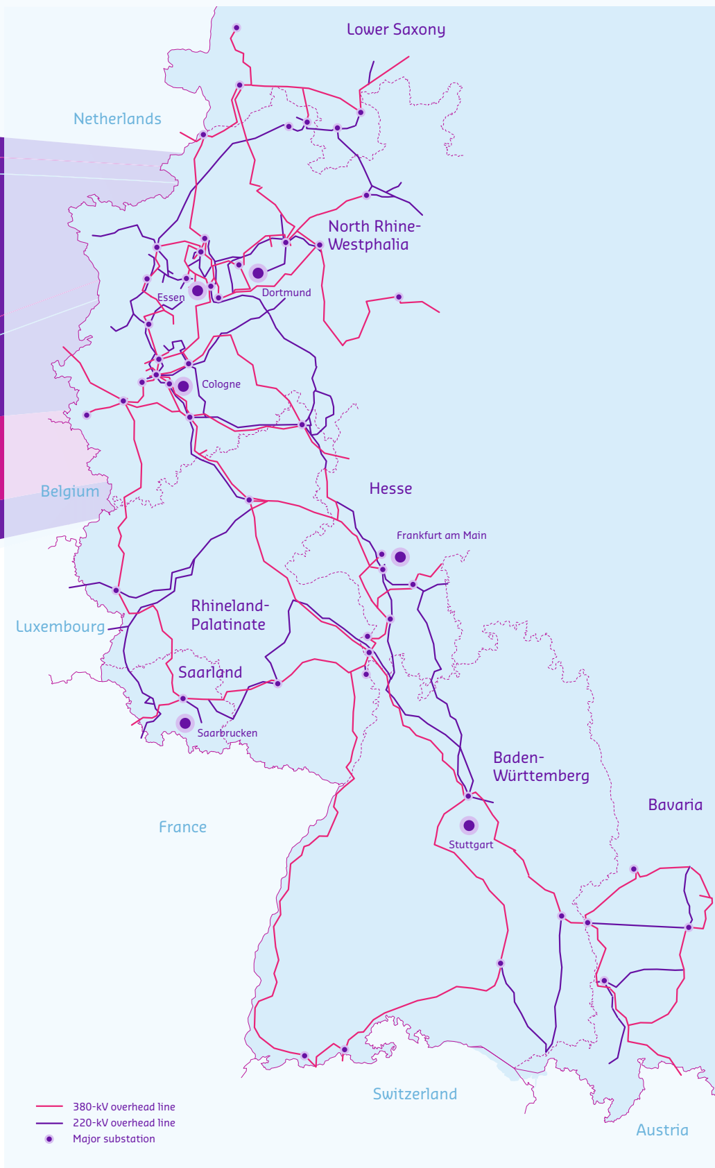
The Amprion 380-/220-kV system
